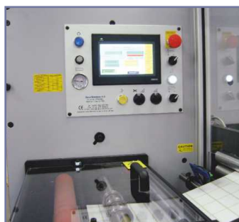
Touch screen control and rotary slitting
