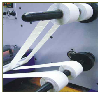
Twin rewinds (air shafts)
