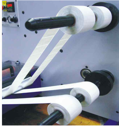
Twin rewinds (air shafts)
