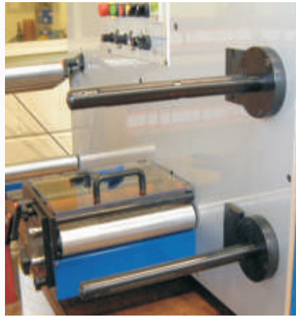
Twin rewinds (air shafts)
